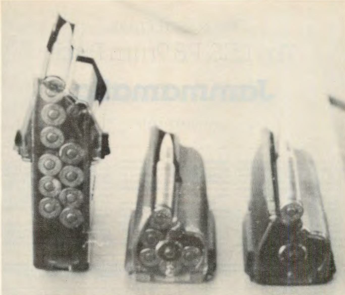
From left: Rotary polycarbonate magazines are 10-round; 5-round; single shot (a plugged 5-round mag.).
